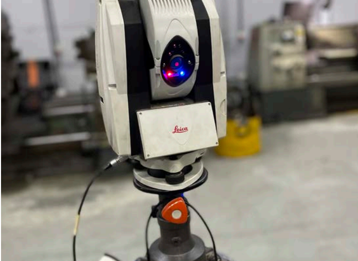
In-Situ Machining measuring is done using Laser Tracker with reference to the sealing surface
